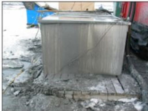
Drill hole 8440M showing overflow of drill fluids. From DNR field report 28 and 29 October 2008.
