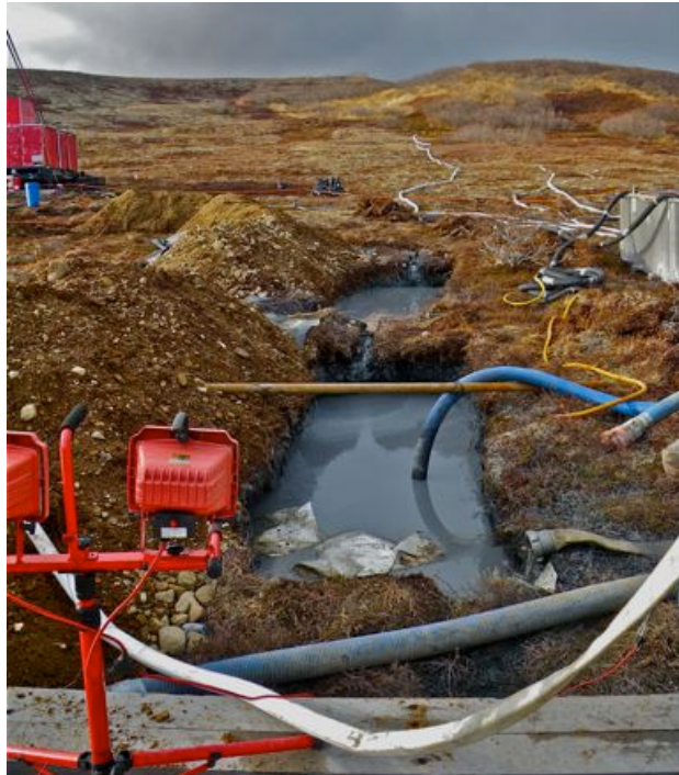
Figure 4. Drill rig sump system at Pebble Limited Partnership Drill Rig #6, South Fork Koktuli River, 22 October 2012. Used drill fluid containing cuttings, additives, and possibly petrochemicals were pumped into an unlined series of five sumps. Heavier materials sink to the bottom, some fluids leach into the ground; remaining fluids are ultimately disposed of on the tundra.
