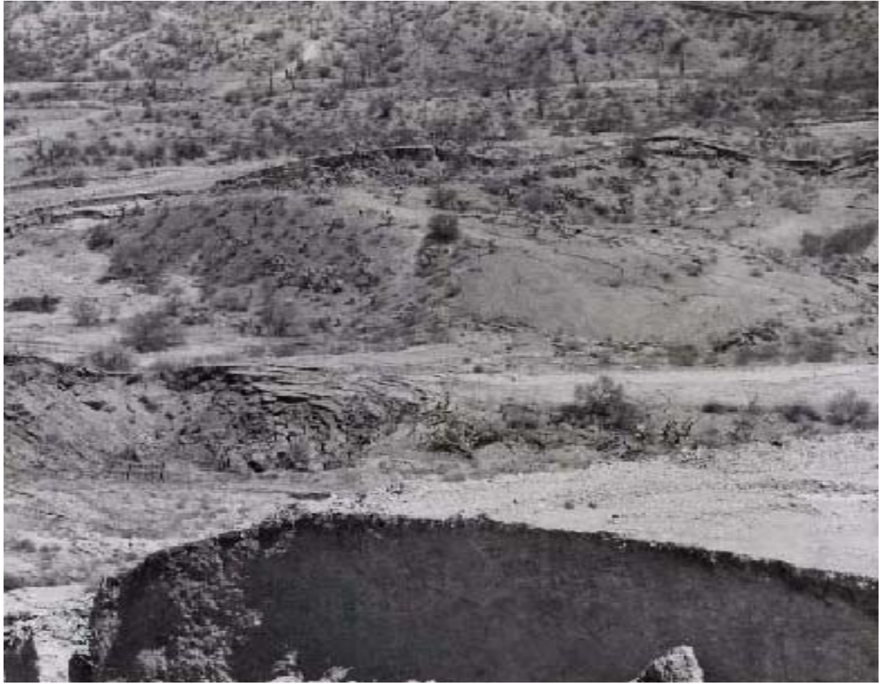
Figure 3: Subsidence due to block caving at the San Manuel copper mine, Arizona
