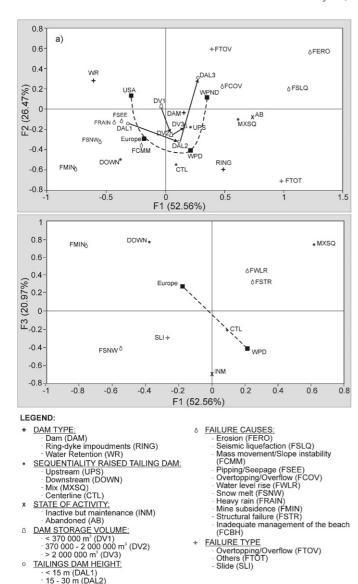
Fig. 5. Projection of attributes and groups of countries onto the first and second plane of correspondence analysis.
