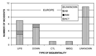
Fig. 4. Distribution of the number of incidents according to type of dam construction and state of activity in the world (above) and in Europe (below). (UPS, upstream; DOWN, downstream; CTL, centerline; MXSQ, mixed construction; ACT, dam active at the moment failure happened; INM and AB, dam inactive at the moment failure occurred, abandoned (AB) or inactive but maintained (INM).
