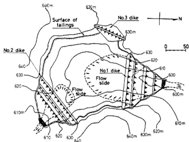
Ishihara (1984) estimated the peak ground acceleration at the dam sites was about 0.15 to 0.25g at the ground surface. Dam No. 1 failed during the main shaking. Dam No. 2, failed about 24 hours after the main shock. The delayed failure of the No. 2 dam was postulated to be due to upward movement of the phreatic surface resulting from liquefaction of the tailings deposits behind the dam (Ishihara 1984).
