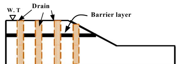
Fig. 17. Stabilizing soil column
