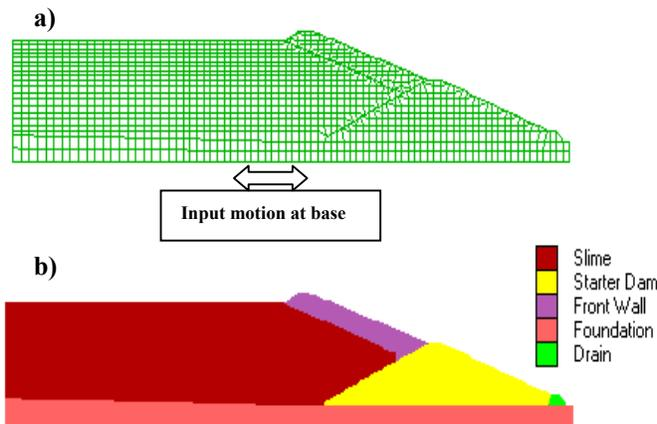
at the Caltech B Station (California Institute of Technology) and normalized to  $a_{max} = 0.15g$  was applied at the base of the model, and is as shown in Fig. 6.
