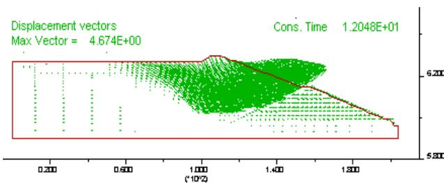
Fig. 13. Distorted grid (3 times magnified for clarity).
